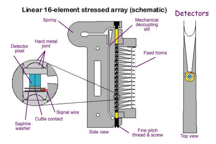
• Self-adjusting joints for homogeneous stress
