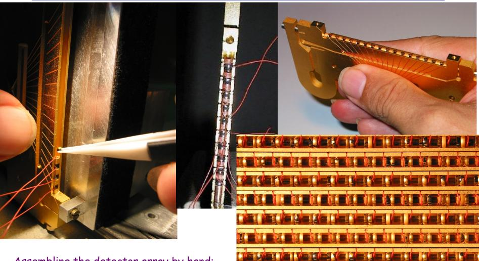
Assembling the detector array by hand: 800 individual pixels
