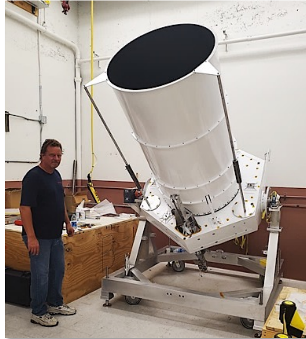
0.9 m f/10 Cassegrain telescope, under-illuminated at high frequencies
