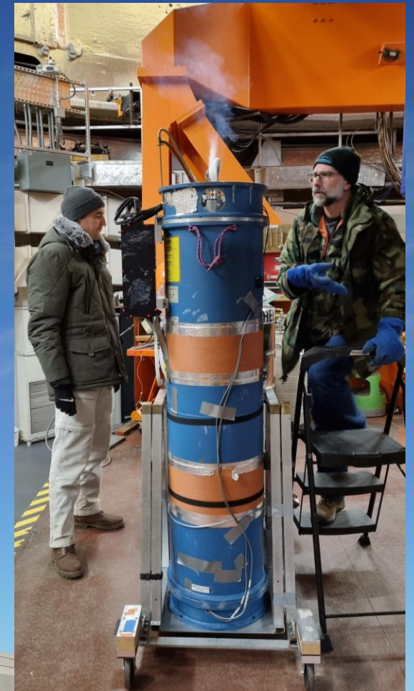
TEXES (Texas Echelon Cross Echelle Spectrograph) 4.5 – 25 \mu\text{m} wavelength region R \approx 50,000 - 100,000
